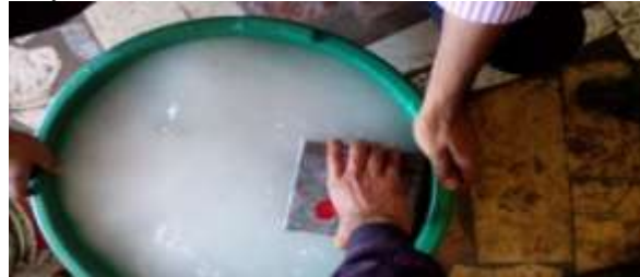
FIGURE 5.6: ALKALINE ATTACK TEST OF CONCRETE CUBES
